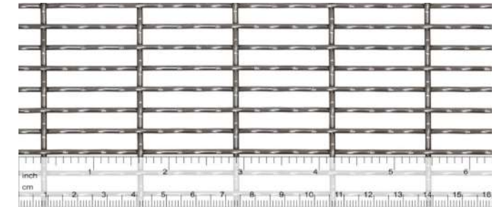
DOKAWELL-MONO 3691 | Weight: 4.2 kg/m 2 | Open area: 70%
